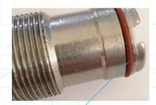
Particular attention needs to be paid to sealing areas ensuring that no damage is present that can compromise the integrity of the O-rings. Delavan strongly recommends the replacement of these O-rings each time the nozzle is assembled.
